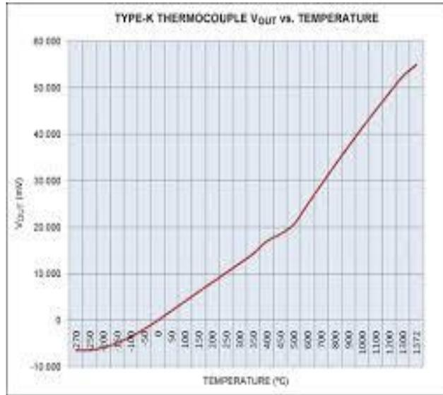
Figure – 1: Voltage Vs Temperature Standard Graph for K-Type Thermocouple
